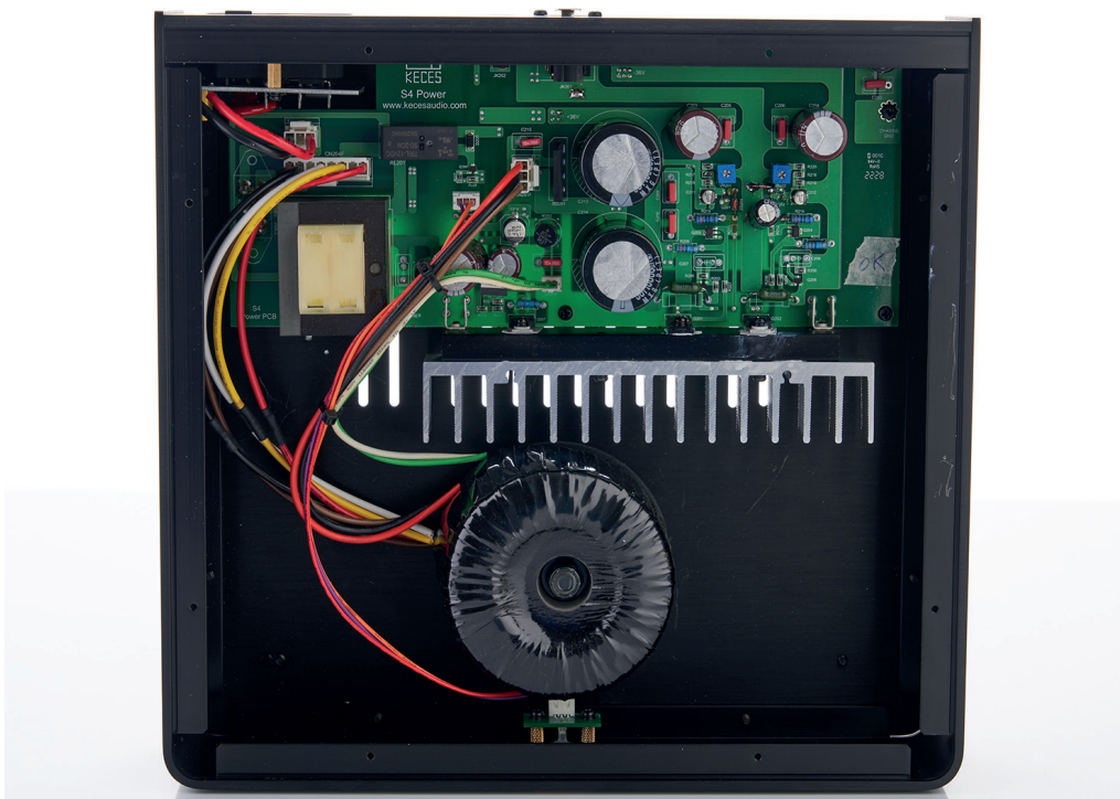
Toroidal power transformer, rectification and filtering were relocated and exiled in a separate housing
