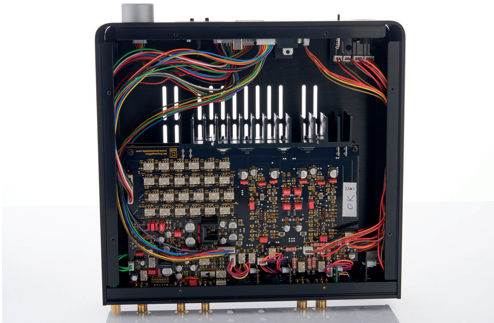
The interior of the preamp captivates with a super-clean design featuring separate SMD boards for the left and right channels in double-mono design, which are arranged piggyback on top of each other
